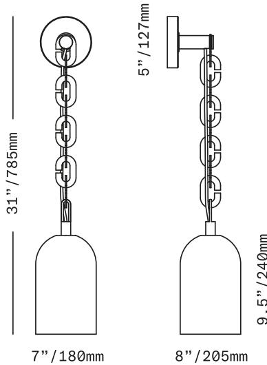
A dome of handblown Czech glass with a frosted finish is suspended on a length of custom brass chain. An exposed, fabric-wrapped electrical cord runs through the chain from the canopy to the glass dome.
