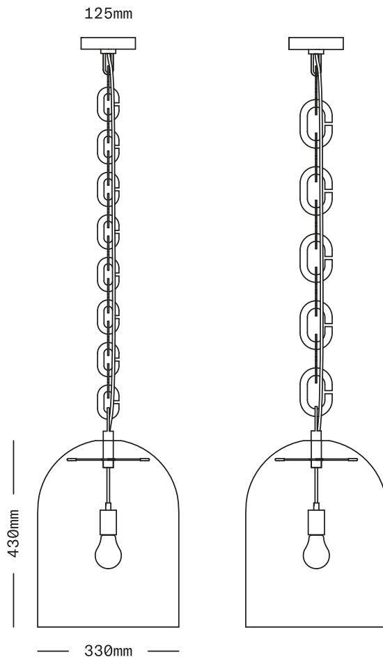
Large domes of handblown Czech glass with a frosted finish are suspended on lengths of oversized brass chains. An exposed fabric-wrapped electrical cord runs through the chain from canopy to light.
