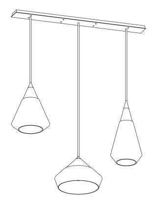
The Linear Multi-Pendant Canopy program is designed to enable multiple SkLO pendants to be suspended from a single 5" (125mm) wide linear canopy. The canopy is available in various lengths, and longer lengths are comprised of multiple sections. This provides the Trade customers with the opportunity to create highly customized SkLO light fixtures. The number of individual pendants and their composition are entirely customizable.
