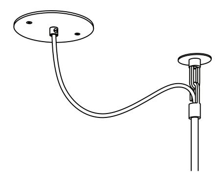
The Swagged Hang-Straight Canopy option enables many of SkLO stem-hung fixtures to be suspended from a location separate from the electrical box while also accommodating all ceiling slopes.
