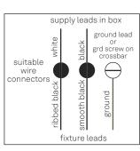
Figure 2. Wiring Diagram
