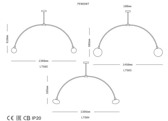
Symmetrical downward curving arms hold glass diffusers of handblown Czech glass. Suspended on a rigid brass tube stem. The glass diffusers are available in three shapes and in both "dipped" glass, featuring the SkLO double-dipped flame-polished mouth and "textured" glass, featuring a soft, frosted finish and subtle sculpted vertical ridges.
