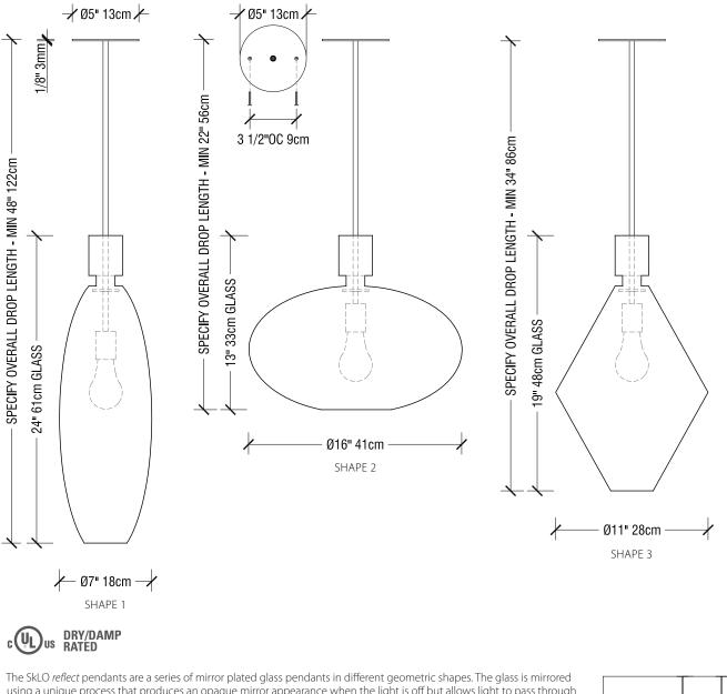
using a unique process that produces an opaque mirror appearance when the light is off but allows light to pass through when on. Each shape has an open mouth at the bottom - the holes are ground flat and polished. The mirrored glass shades rest atop a disc at the end of the rigid brass stem - light bulbs are accessed by either reaching through the open hole or by carefully raising the glass up over the bulb.
