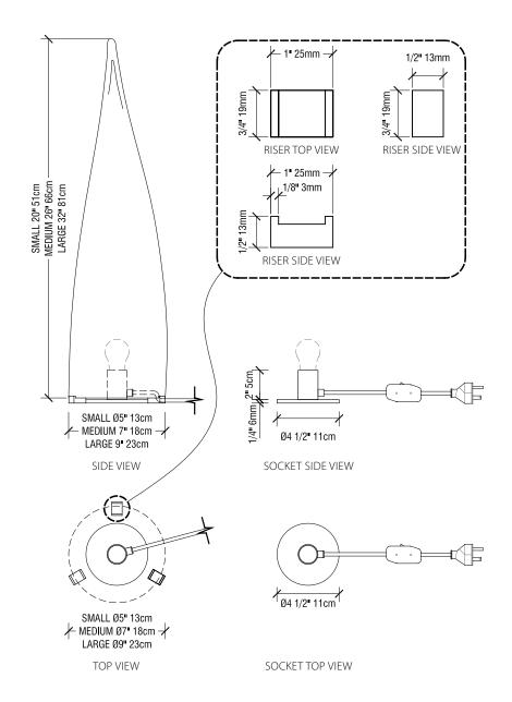
The SkLO *kin* light combines a large conical piece of handblown glass as a diffuser with a separate brass socket. The glass has an opaque color at the base which fades to clear at the top. Glass is available in three sizes. The polished bottom edge of the glass rests atop three loose solid brass risers (to be arranged evenly around the circumference of the base of the glass as shown) to allow the cord from the light socket to pass beneath the glass.
