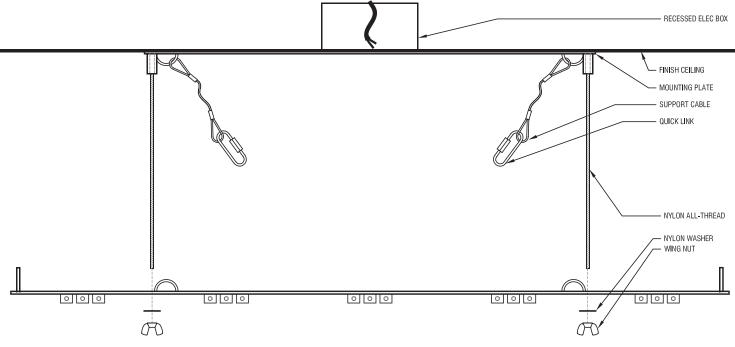
Figure 3. Install nylon all-thread rods into mounting plate and slide canopy up over rods
