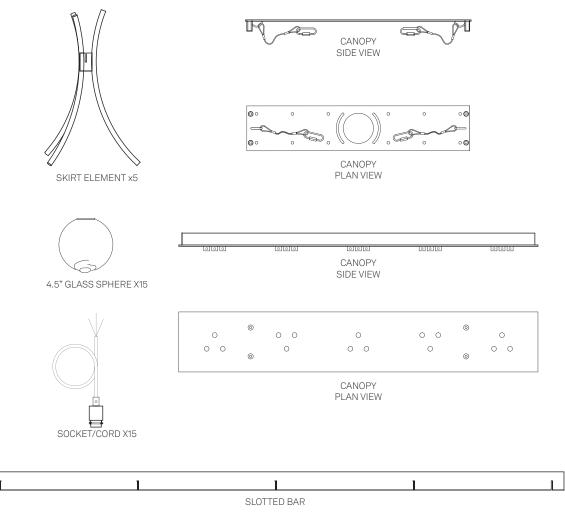
Figure 1. Parts of the Light Fixture Assembly
