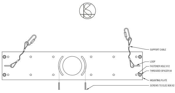
Figure 2. Install mounting plate
