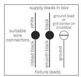
Figure 7. Wiring Diagram
