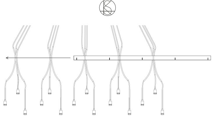
Figure 6. Attach brass bar to individual "skirt" elements
