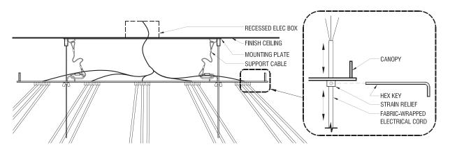
Figure 5. Attach support cable to canopy ... raise canopy, remove nylon rods and fasten canopy to mounting plate
