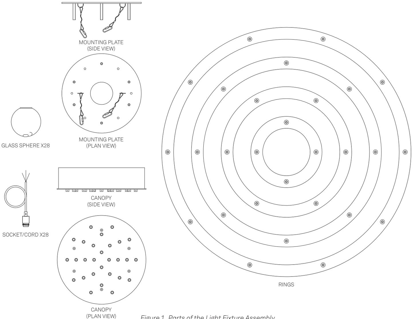
Figure 1. Parts of the Light Fixture Assembly
