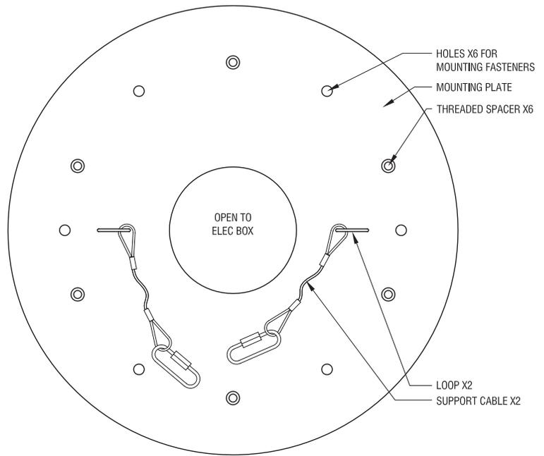
Figure 2. Install mounting plate
