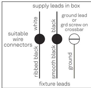
Figure 7. Wiring Diagram
