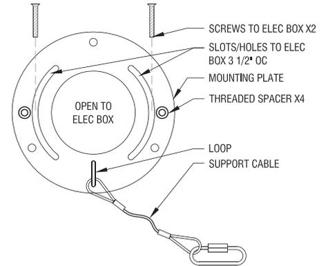
Figure 2. Install mounting plate
