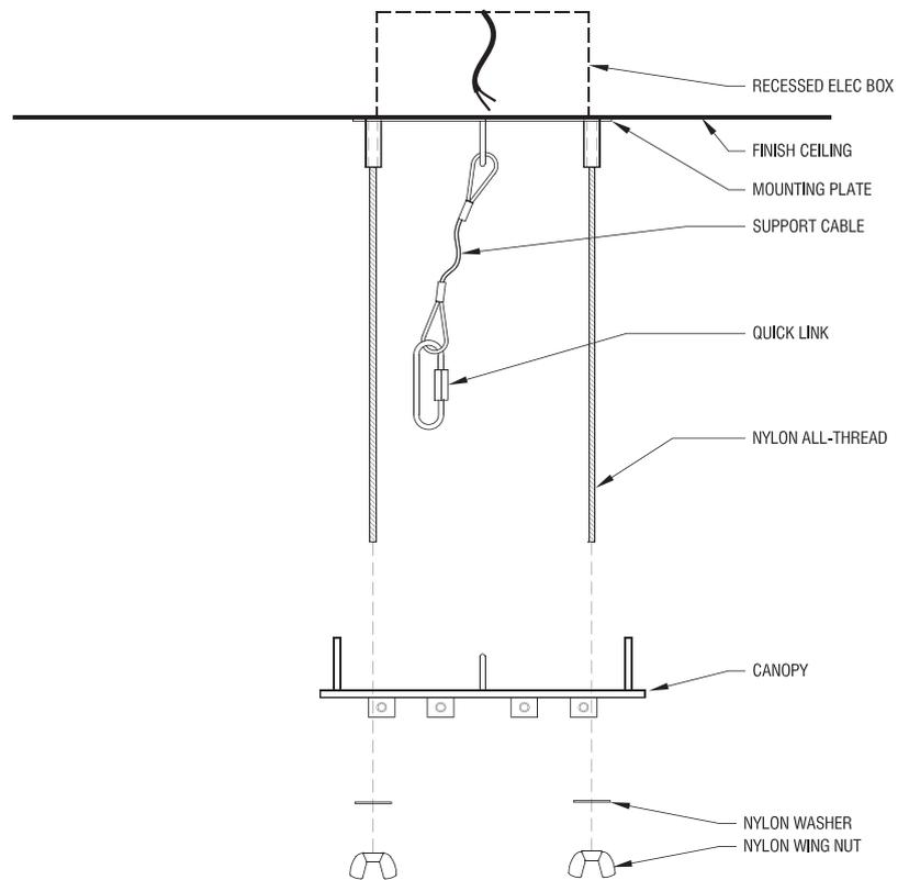
Figure 3. Install nylon all-thread rods into mounting plate and slide canopy up over rods
