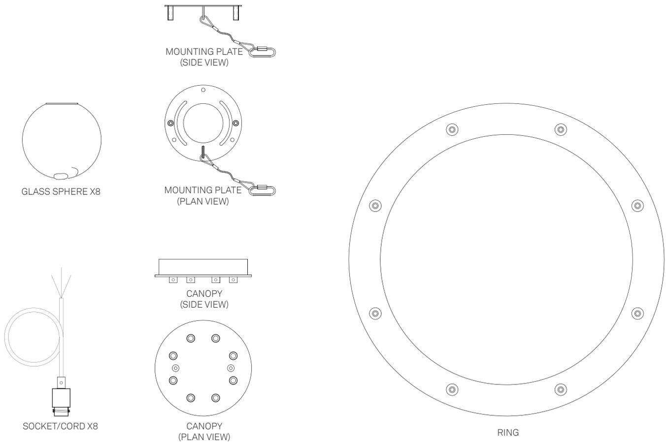
Figure 1. Parts of the Light Fixture
