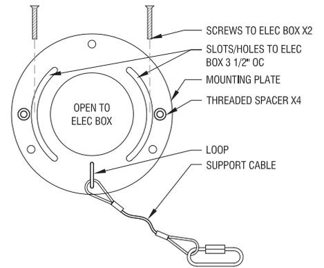
Figure 2. Install mounting plate
