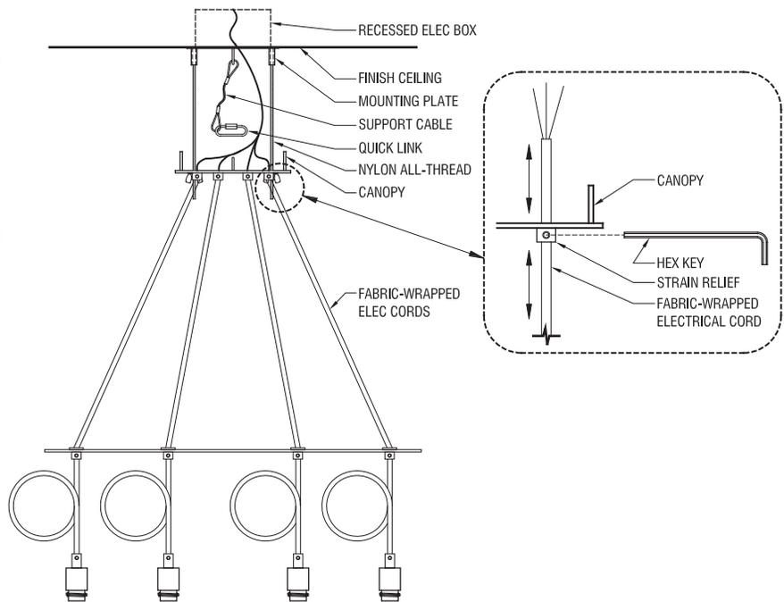
Figure 5. Leveling the fixture
