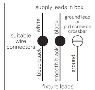
Figure 6. Wiring Diagram
