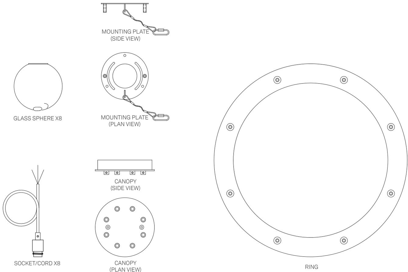
Figure 1. Parts of the Light Fixture
