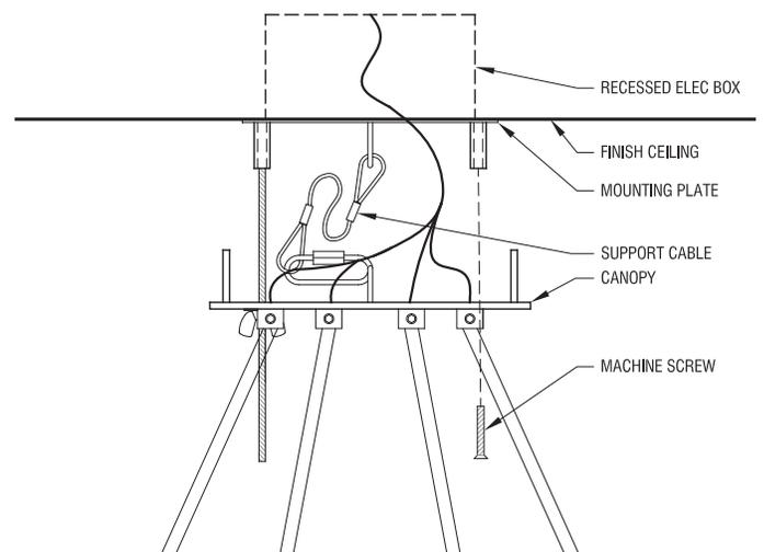
Figure 7. Fasten canopy to mounting plate
