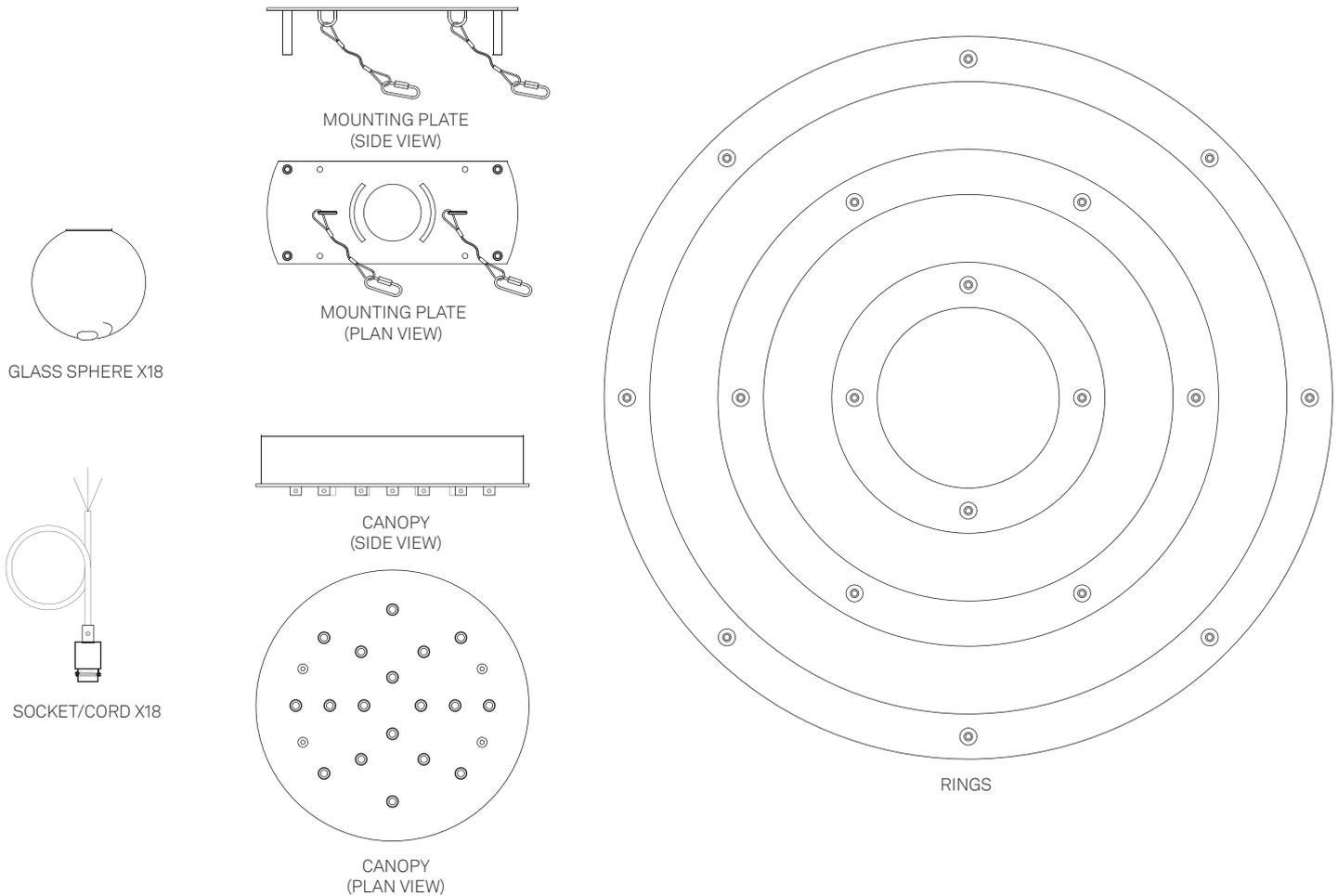
Figure 1. Parts of the Light Fixture Assembly
