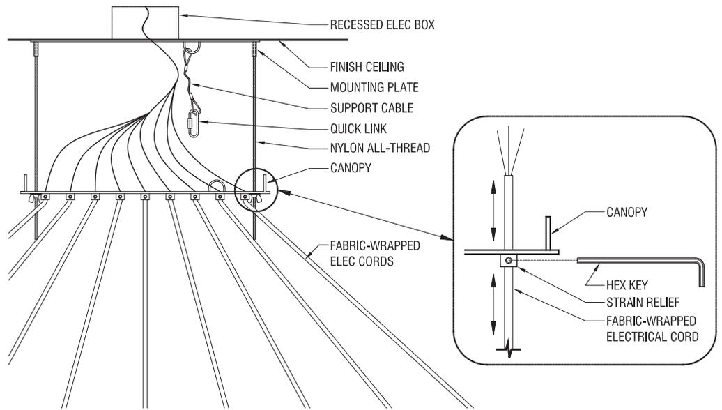
Figure 5. Wiring the fixture / adjusting and checking level
