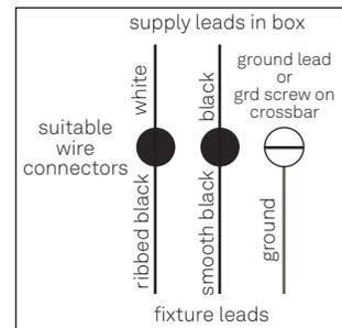
Figure 6. Wiring Diagram
