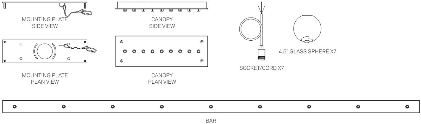
Figure 1. Parts of the Light Fixture Assembly
