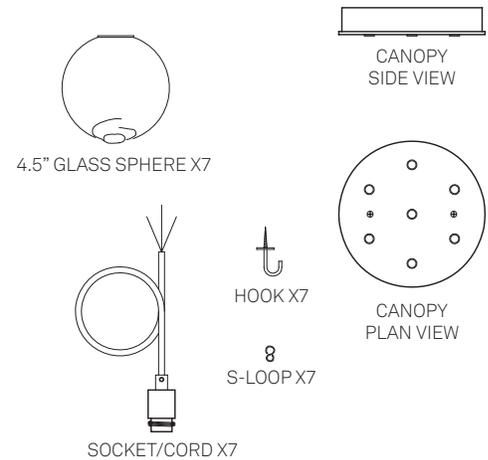
Figure 1. Parts of the light fixture assembly
