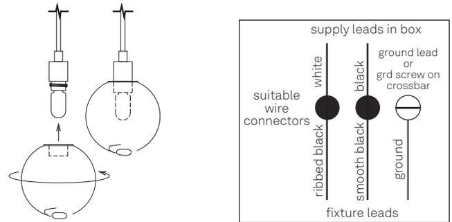
Figure 4. Install glass spheres by threading onto brass sockets
