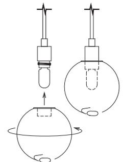
Figure 4. Install glass spheres by threading onto brass sockets
