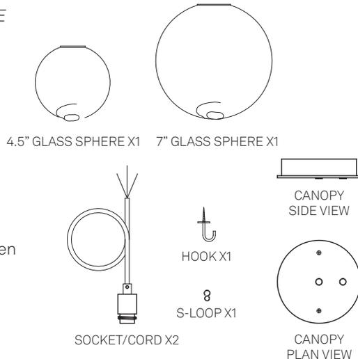
Figure 1. Parts of the Light Fixture Assembly
