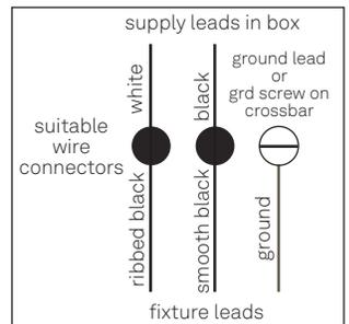
Figure 2. Wiring Diagram
